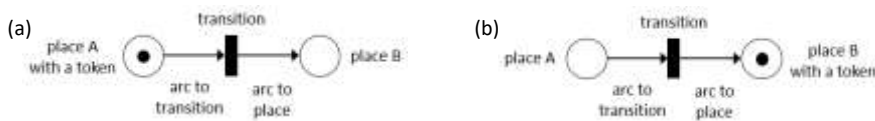
Figure 9 - Example of Petri net diagram (a) before and (b) after the transition is fired.
