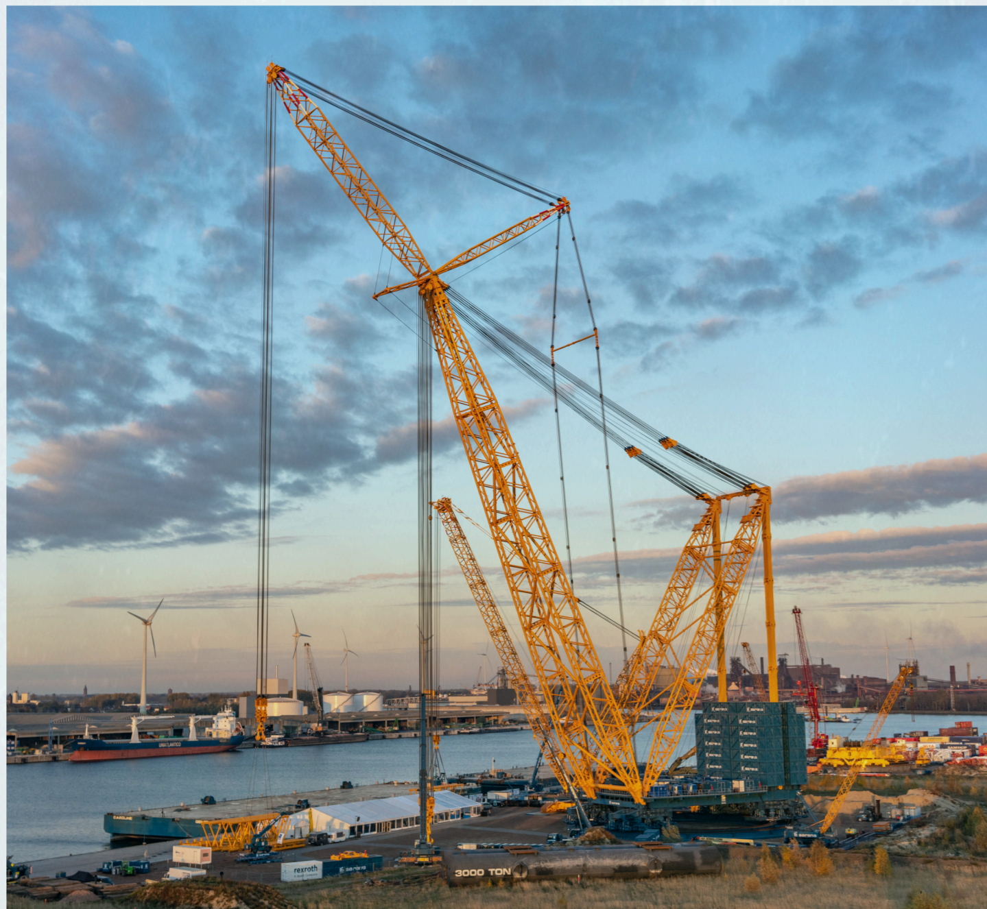
Image Credit: Sarens - SGC-250, the Sarens Giant Crane nicknamed 'Big Carl' by the Port of Ghent
